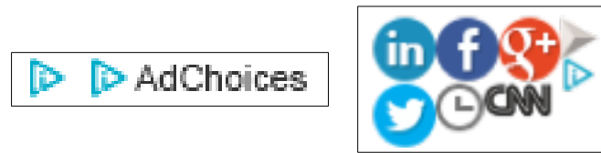
Figure 3.13: Image sprites of the AdChoices logo. Image-sprites are sets of images stored in a single file, and segmented using CSS rules. For example, the left sprite allows to smoothly switch from the icon to the full logo on hover. The right sprite is used by cnn.com to load a variety of logos used on the page in a single request.
