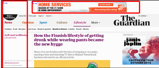
(c) Attack C3 (Universal): The publisher overlays a mask on the page to generate unreasonably large boxes and disable the ad-blocker.
